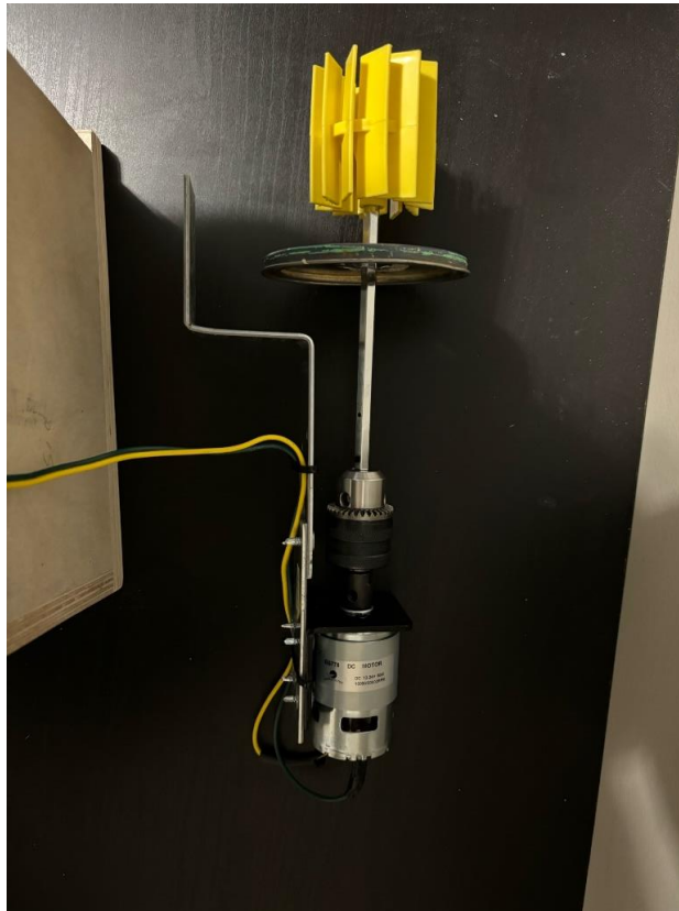
Figure 4: Impeller-Lid-Rod-Motor-Bracket Connection
