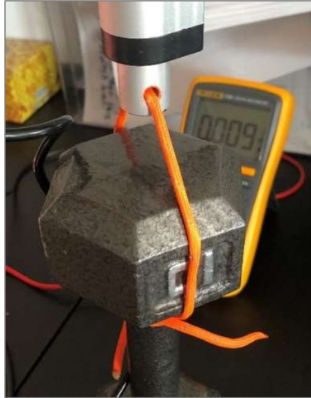
Figure 21: Linear Actuator with 10 lbs. Load Attached
