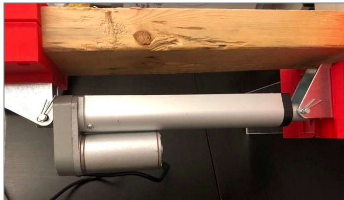
Figure 8: Installed linear actuator
