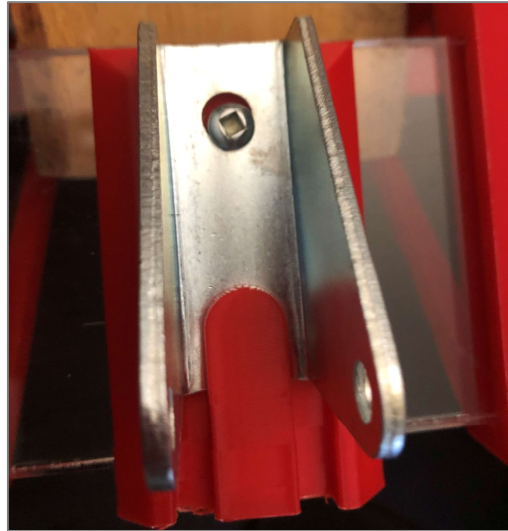
Figure 5: Lower linear actuator mount bracket
