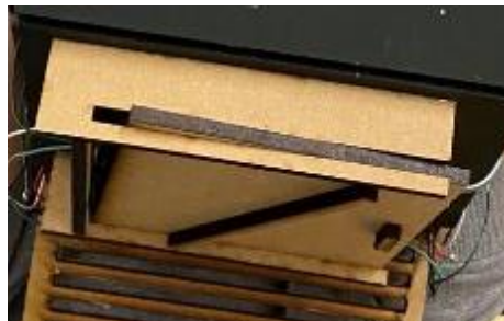
Figure 5.4: Electronics compartment with the sliding door in place
