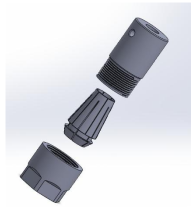
Figure 2.5: Exploded View of the Assembly
