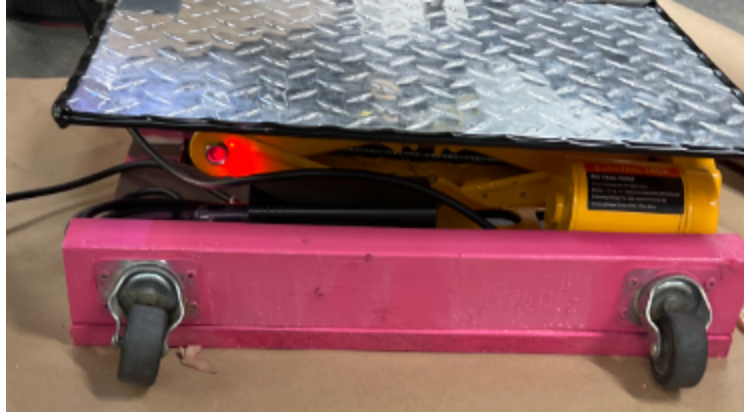
Figure 9: Portability - Wheels are attached with the step
