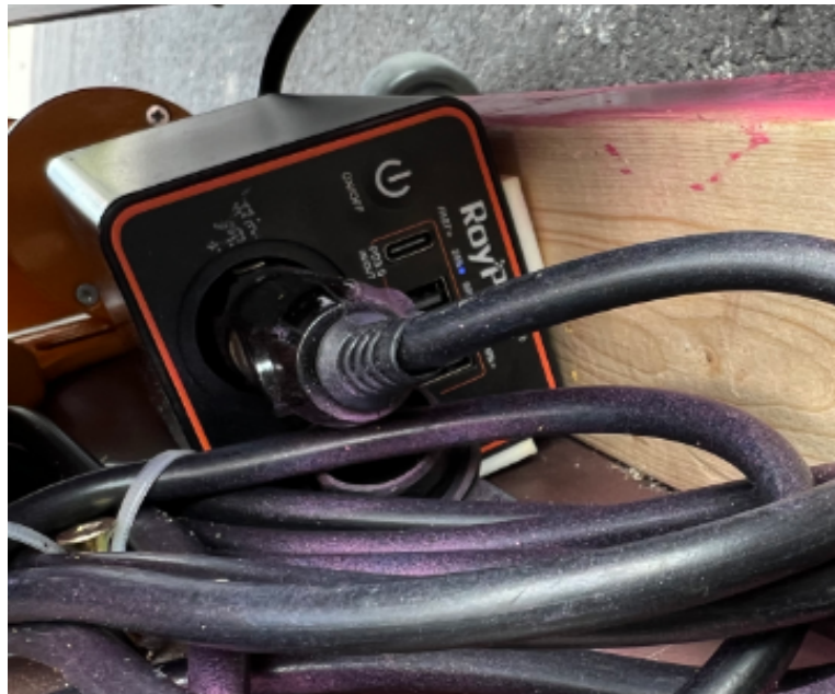
Figure 6: Making sure the cigarette lighter output is connected to the battery, the power button is the top right button.
